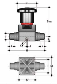
Compact diaphragm valve with male ends for solvent welding, metric series
