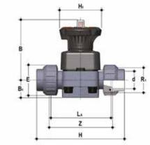
**DKUIV**DIALOCK® diaphragm valve with female union ends for solvent welding, metric series
